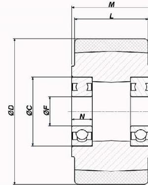
**POLYURETHANE WHEELS WITH SINGLE BALL BEARING**
